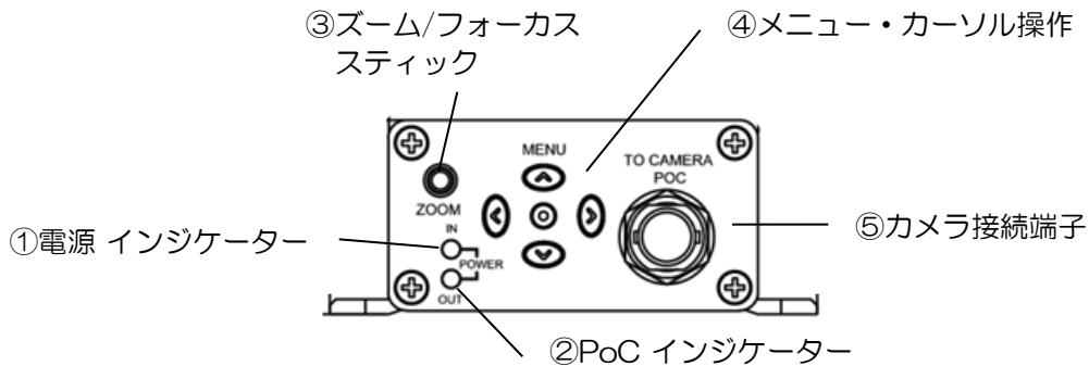
PoC : Power Over Coax (同軸線電源供給)
